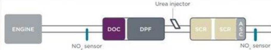
Figure 1. EPA 2010 aftertreatment system layout.
